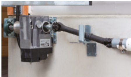
Fixed motor mounting with gimbal for coupling with the sail
